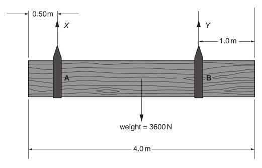
The weight of the beam is 3600 N and its length is 4.0 m. The strap **A** is positioned 0.50 m from one end of the beam and the strap **B** is positioned 1.0 m from the other end.
