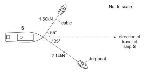
The ship is travelling at a constant velocity. The tensions in the cables and the angles made by these cables to the direction in which the ship travels are shown in the figure above.
