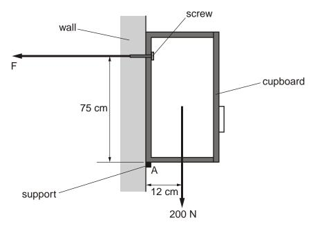
The total weight of the cupboard and its contents is 200 N. The line of action of its weight is at a distance of 12 cm from **A**. The screw securing the cupboard to the wall is at a vertical distance of 75 cm from **A**.
